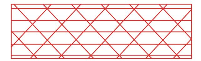
Waco's reinforced gummed tapes are made by laying fibreglass threads within a laminate of two layers of strong Kraft paper, suitably coated on one side with a special glue.
